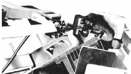
Figure 7. Blade Backup Bearing
