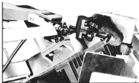
Figure 8. Blade Backup Bearing
