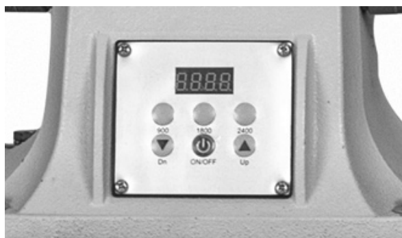
Figure 4 – Control buttons from left to right; top row: 900 RPM, 1800 RPM, and 2400 RPM; bottom row: Dn – “Down”, ON/OFF, and Up.
