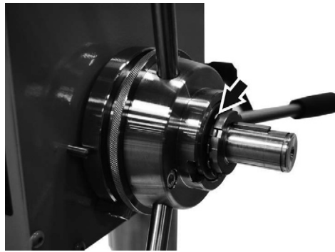
Figure 12 – Adjusting the feed switch.
