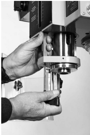
Figure 19 - Removing the depth stop rod.
