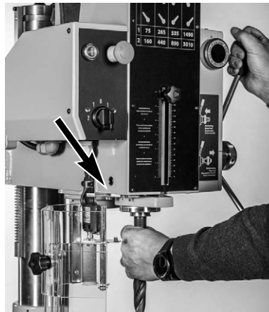
Figure 14 - Automatic drill ejection.
