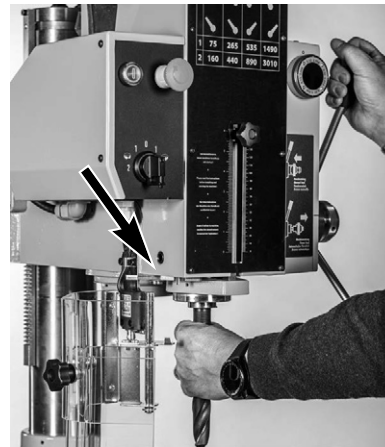
Figure 14 - Automatic drill ejection.
