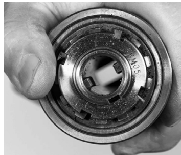
Figure 20 - Nut for adjusting the play of the quill.
