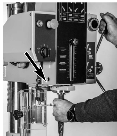
Figure 14 - Automatic drill ejection.
