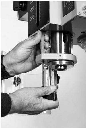
Figure 19 - Removing the depth stop rod.
