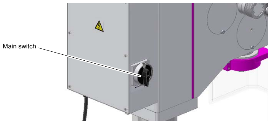
Img. 1-2: Main switch
