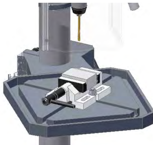
Img.4-1: seats for clamping blocks
