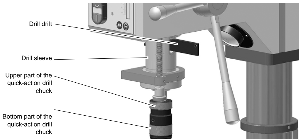
Img.4-8: Disassembly using the drill drift
