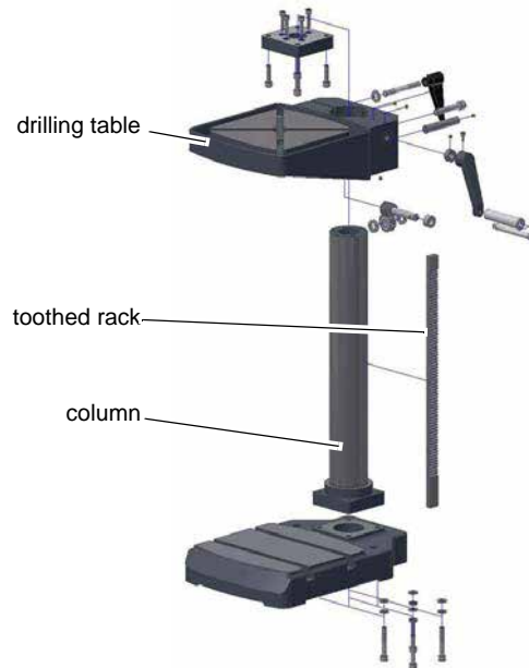
Fig.3-2: Assembly drilling table B24H (Vario)
