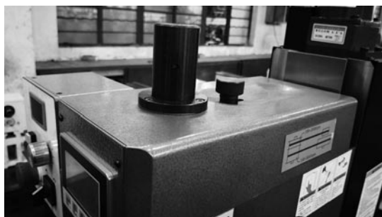
Figure 23 – Gear cover replaced.
