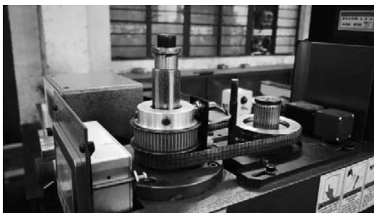
Figure 15 – Spindle belt and gearing.
