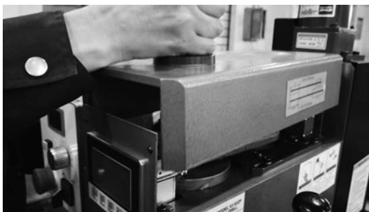
Figure 14 – Gear box cover removal.
