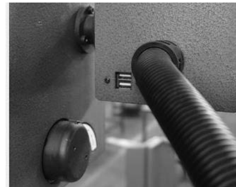
Figure 11 - With two USB sockets, can supply power.
