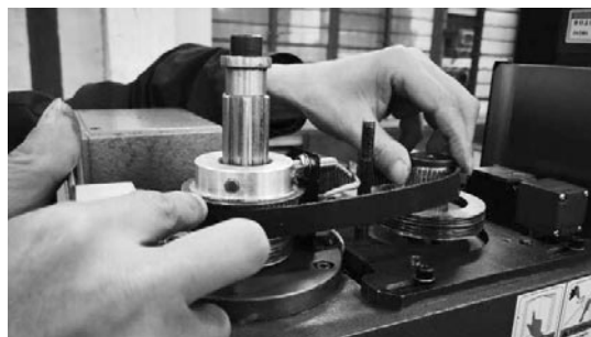
Figure 19 – Shifting belt to upper low-speed gear.
