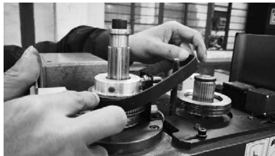
Figure 18 – Shifting belt to upper low-speed gear.
