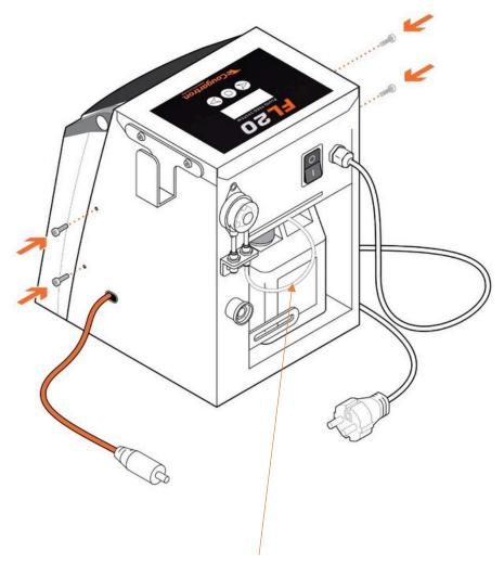
1. The short fluid line needs to be put into the fluid container.
